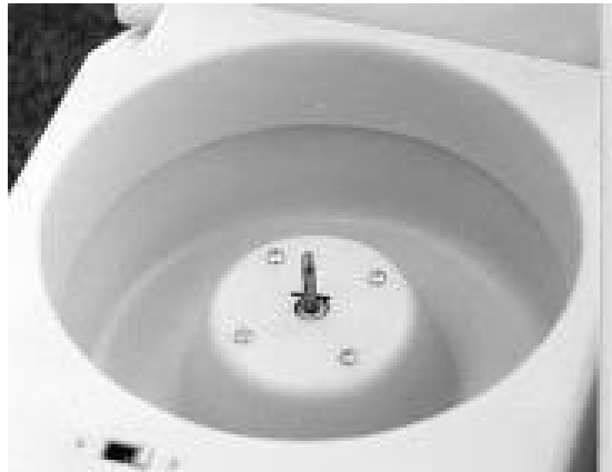
Figure 1. Chamber and motor shaft
